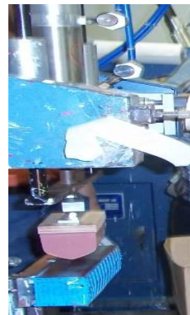
Shown here is a boxcar being pad printed with a road name, car number, or other fine detail.
