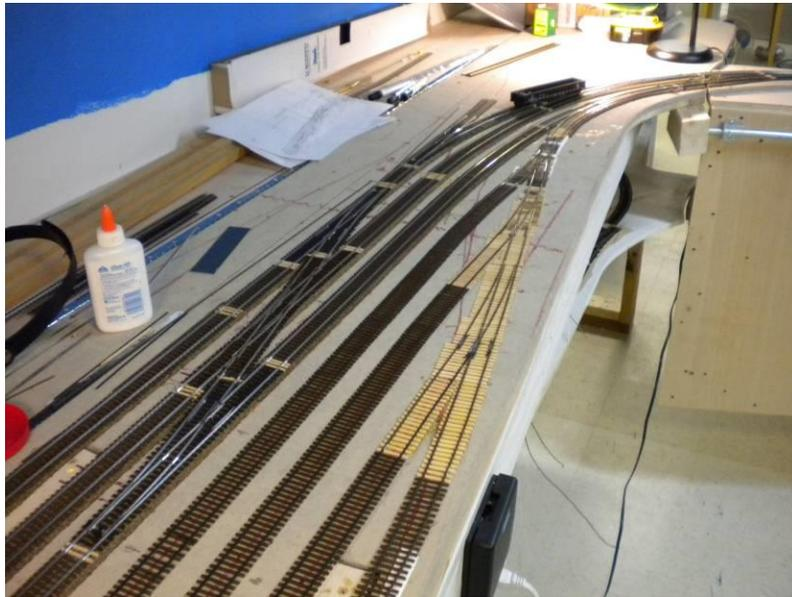
The photo above shows the Cornwall yard raised and being supported by one of the three struts. This hinged section allows maintenance access to the staging yard below as well as the wiring for Cornwall.
