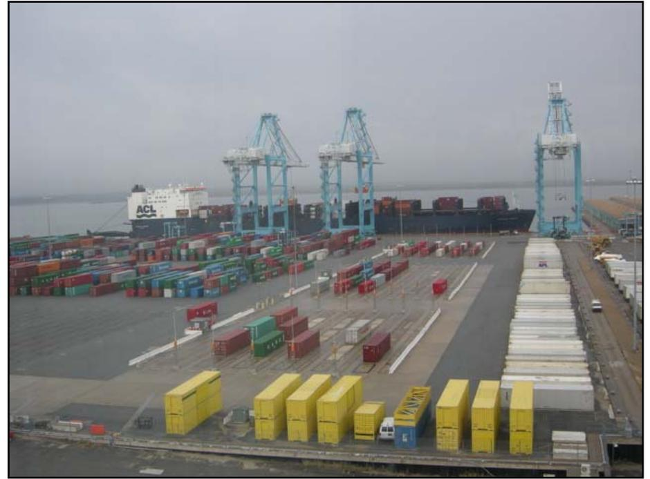
*This view is facing east where we could see the entire yard. The yellow containers at the bottom of the photo are the port radiation detectors. The ACL ship at the dock was a standard 900 foot variety. The gantry cranes remove containers from the ship and place them on the dock next to the ship. Then straddle cranes pick the containers up for placement somewhere in the yard or directly on one of the trains being made up.*
